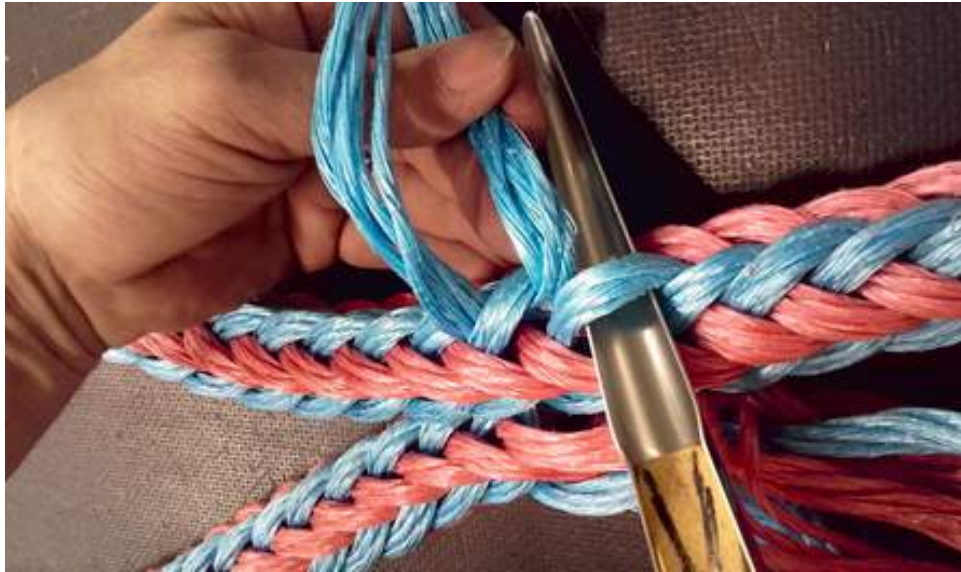
Figure no. 21: Lacing both "Z" strands
