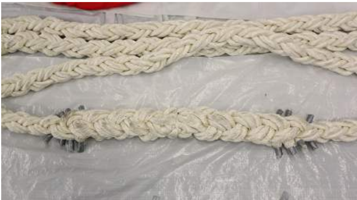
Figure no. 18: Finished splice
