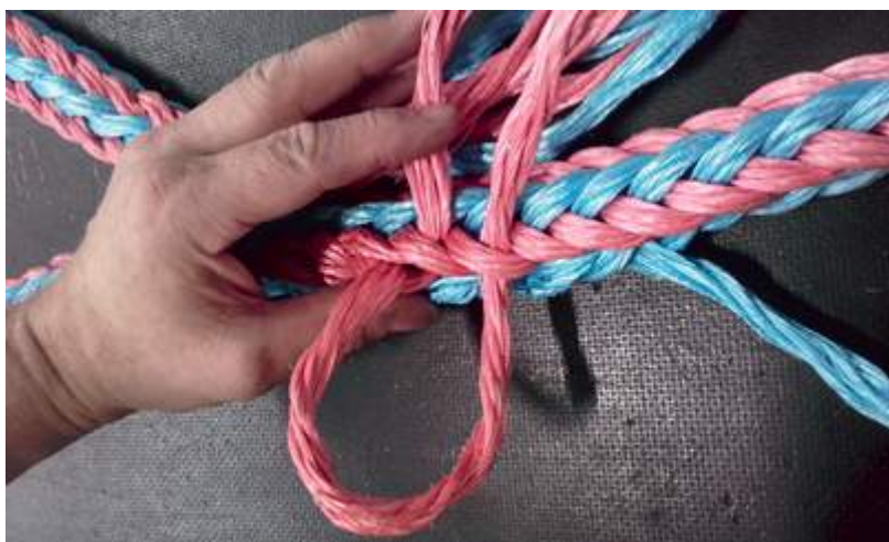
Figure no. 23 c): Tucking the "S" strands
