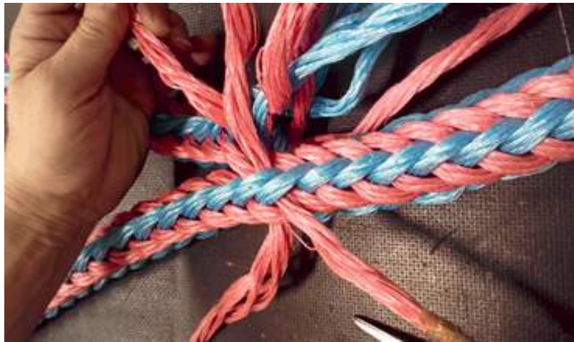
Figure no. 23 b): Tucking the "S" strands
