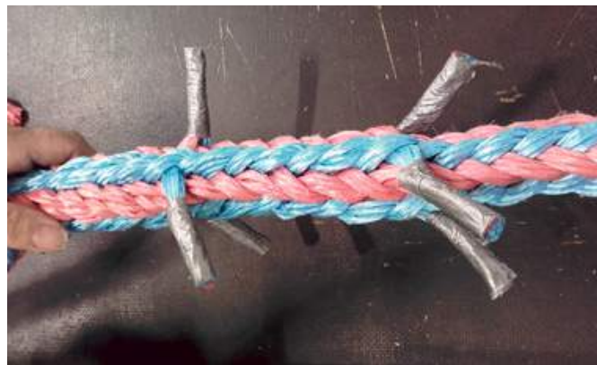
Figure no. 25 a): Finished splice
