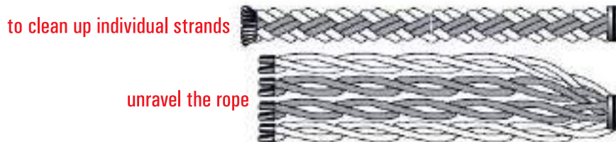
Figure no. 14: 8-strand braided ropes (end-to-end) - step 3
