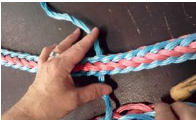
Figure no. 20: Lacing the “Z” strand through the middle of the rope
