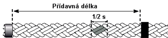
Figure no. 6: Marking the length of splice
