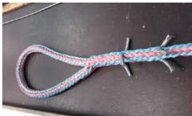
Figure no. 25 b): Finished splice
