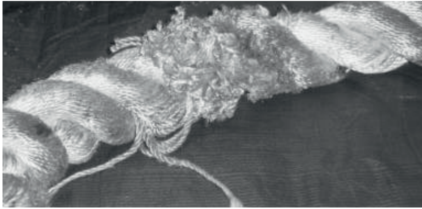
Figure no. 6 c): External abrasion - Localized external abrasion 2
