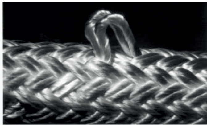
Figure no. 9: Localized external abrasion 1
