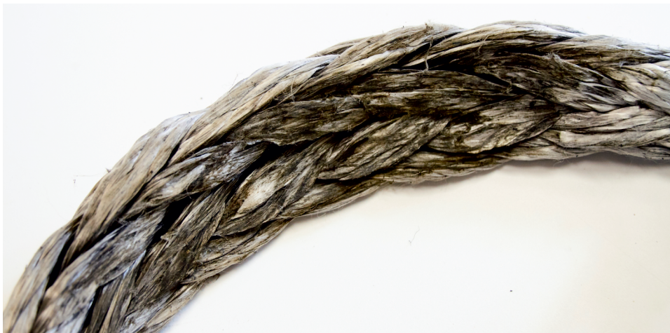
Figure no. 7: Burn and melting from external abrasion
