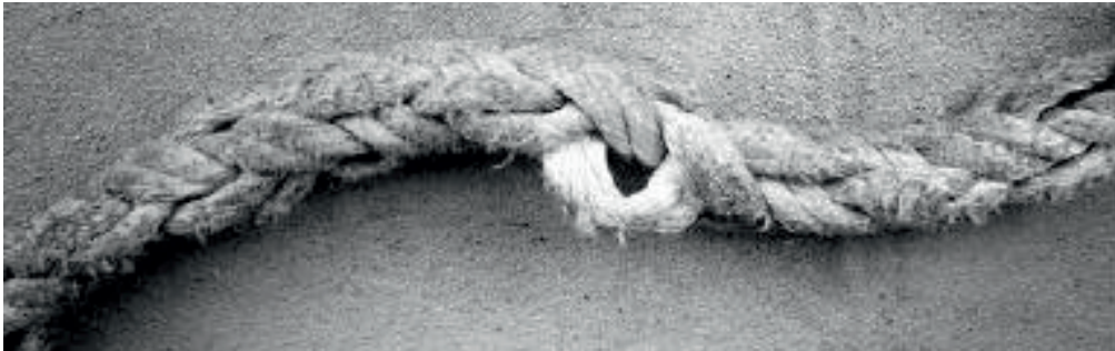
Figure no. 5: Matted internal yarns (exposed stands reveal internal matting)
