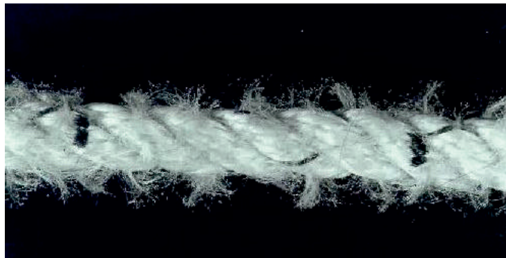
Figure no. 14: UV degradation of PP rope
