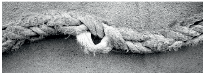
Figure no. 10: Localized external abrasion 2
