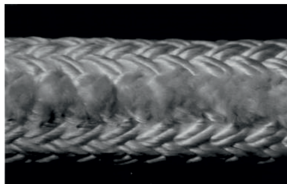
Figure no. 6 b): External abrasion - Localized external abrasion 1
