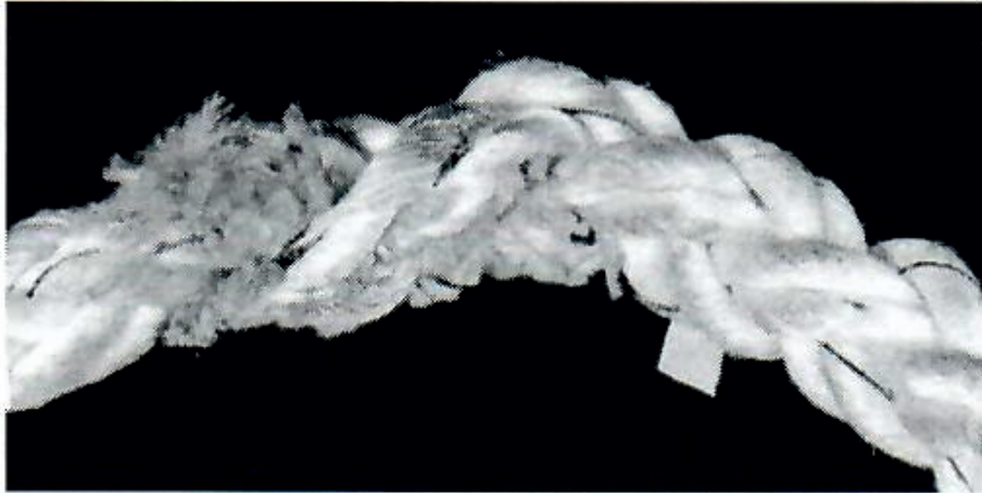
Figure no. 8: Localized external abrasion
