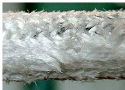
Figure no. 15: Melting of fibers
