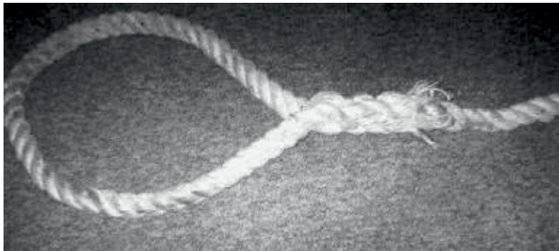
Figure no. 11 a): damage of splicing - 3-strand splice of poor quality
